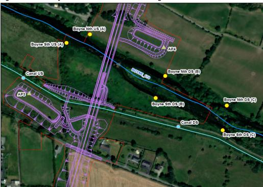
Figure 7.1: River Boyne Construction Phase Monitoring Locations
