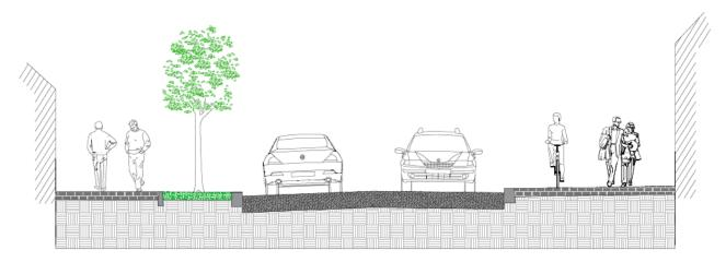
Figure 4.21: Typical Proposed Cross Section – Existing N2 Chapel Street (Section at Ch. 35)
