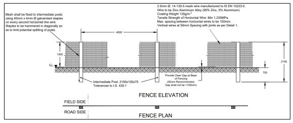
Figure 4.33: Timber Post and Tension Mesh Fence (Taken From TII CC-SCD-00320)
