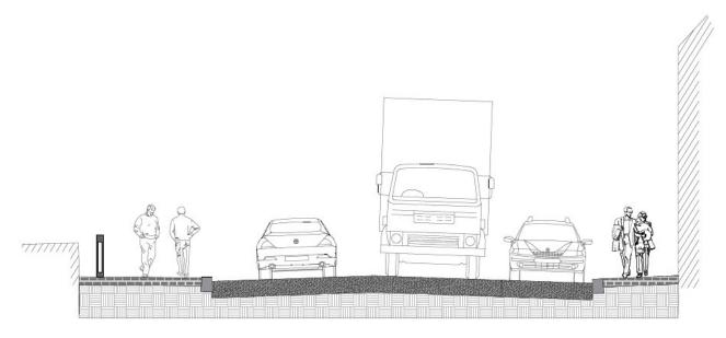
Figure 4.28: Typical Proposed Cross Section - N51 Main Street East (Section at Ch. 70)
