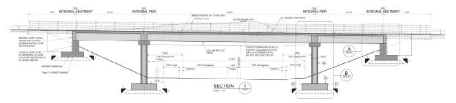
Figure 4.12: Typical Arrangement of the Overbridges
