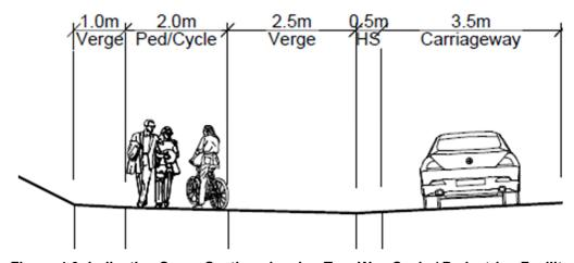
Figure 4.6: Indicative Cross-Section showing Two-Way Cycle / Pedestrian Facility
