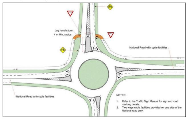
Figure 4.7: Recommended Arrangement for NMU Crossings at Roundabout Junctions
