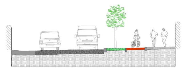
Figure 4.24: Typical Proposed Cross Section – Existing N2 South (Section at Ch. 850)
