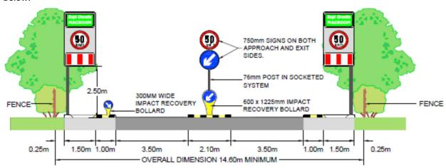
Figure 4.8: Illustration of Type B Gateway
