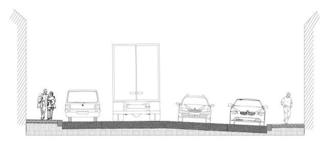
Figure 4.26: Typical Proposed Cross Section – N51 Main Street West (Section at Ch. 180)
