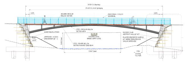
Figure 4.13: Proposed Span Arrangement of the Shared Use Cycle and Pedestrian Bridge
