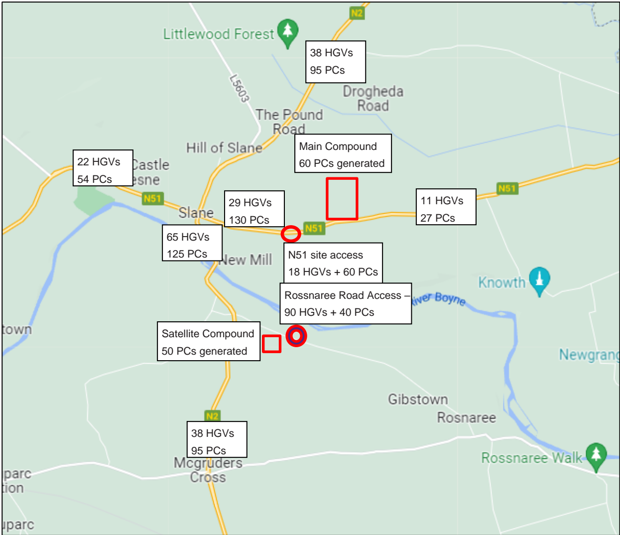
Figure 5.20: Non-Earthworks HGV and PC Trips
